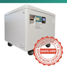
HAPS VRP is a cost-effective three phase precision AC voltage regulator with inbuilt Healthy Automatic Phase Selection (HAPS) system which selects the best incoming voltage phases, ignores incoming neutral and provides a stabilized single-phase output with a fresh grounded neutral. This ensures maintenance-free operation of electronic equipment over a wide range of input voltage range even in situations of phase loss and broken input neutral.
